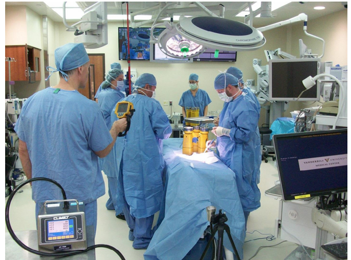
Fig 2. Picture of mock surgical procedure. The multidisciplinary team consisted of a surgeon, nurse, engineers, industrial hygienist, and microbiologist to provide input on the different perspectives of the research project. The same core team performed the mock surgical procedure and testing at all sites and used a steak to cut with an electrocauterization device to simulate the particles generated in actual cases.
